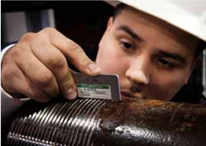
Mercury Threading, one of Houston's processing companies, specializes in cutting threads. Today José Juárez is working the night shift – here he is checking the thread on an oil-drilling pipe.
