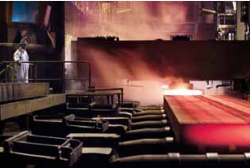
A few meters away the flame cutting machine is cutting the concast into slabs.
