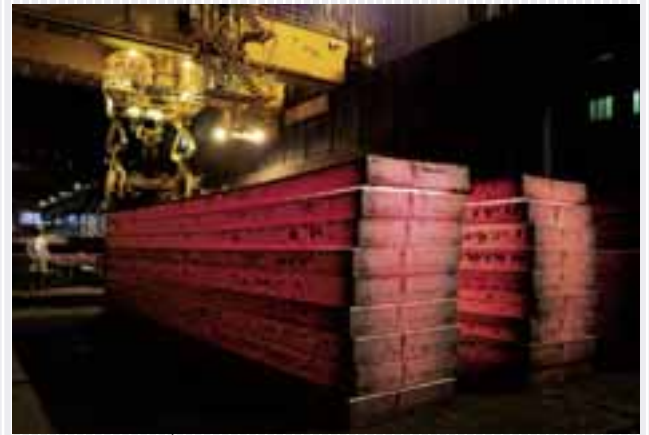
In the slab store, each slab is signed: the character and numerical code enables precise tracking at all times.
