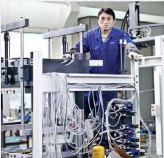
Technician Wang Hongxiang is working on the mold clamping unit of the 250 ton machine – this is the best-selling model.
